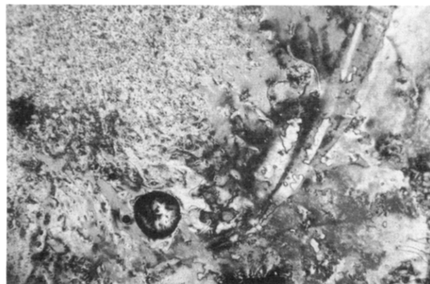
Figure 1. Polarized light micrographs of polymer [N5Cu][P10]: (a) at 220 °C, (b) nematic texture obtained by the addition of bis[ N -(4'-ethoxyphenyl)-4-[[[(decyloxy)benzoyl]oxy]salicylaldiminato]copper(II) taken at 224 °C.
